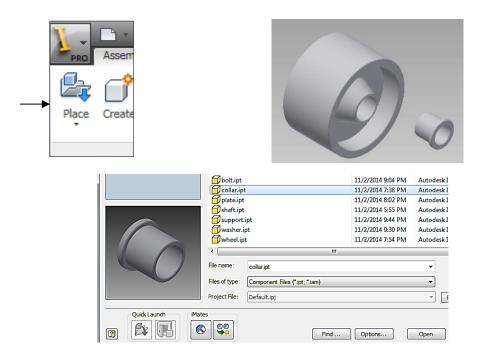
Click *Constraint*. Again, the Type is *Mate*. For Selection 1, choose the right face of Wheel. For Selection 2, choose the left surface on Collar. The Solution is set to *Mate*. Click *Apply*.
