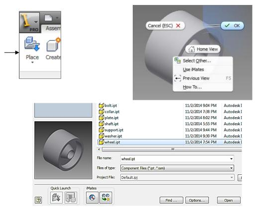
2. Next, insert the Sleeve component. Click *Place* > click on the Collar component >left click anywhere to place the component in the assembly. Click *Constraint*. Again, the Type is *Mate*. For Selection 1,
