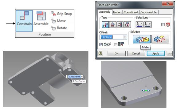
Constrain the left side of Support to the front side of Plate in the same fashion. The Solution is set to *Flush*. Do the same for the back of Support and the right of Plate, as shown in the figures. Click OK when done.
