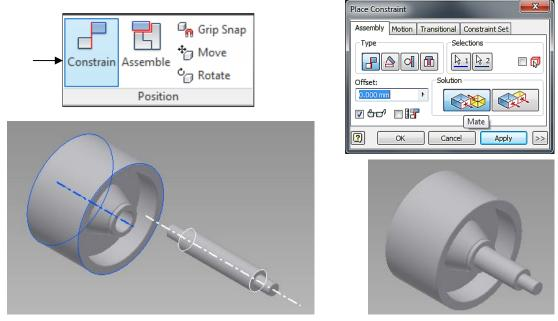
Constrain the Center Point (origin) of the assembly and the Center Point (origin) of Shaft. The Solution is set to *Mate*. Click *Apply*.
