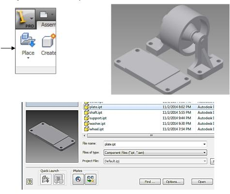
Click *Constraint*. For Selection 1, choose the bottom face of the support. For Selection 2, choose the indentation on the Plate component. The Solution is set to *Mate*. Click *Apply*.
