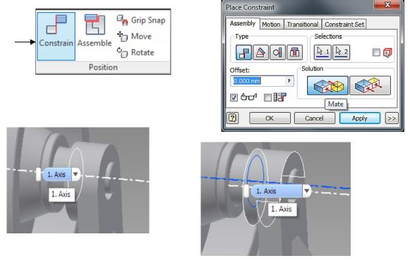
Constrain the (origin) of the assembly and the Center Point (origin) of Shaft. The Solution is set to *Mate*. Users may need to click Flush to align the normal vectors of the 2 surfaces. Click *Apply*.
