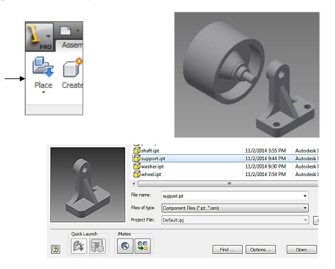
Click *Constraint*. For Selection 1, choose the right face of Shaft. For Selection 2, choose the left surface on Support. The Solution is set to *Mate*. Click *Apply*.
