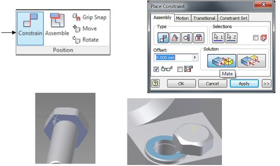
Next, constrain the outer surface of the Bolt shaft to the inner surface of the hole of the Support. For Selection 1, click the axis of the Bolt shaft. For Selection 2, click the axis of the hole of the Support. The type is *Mate* and the Solution is also *Mate*. Click Apply. Click *OK* when done.
